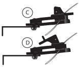
super lines to keep the line from slipping through the pad (E). (Slipping line can damage the pad as well as the pin in the center of the pad).
