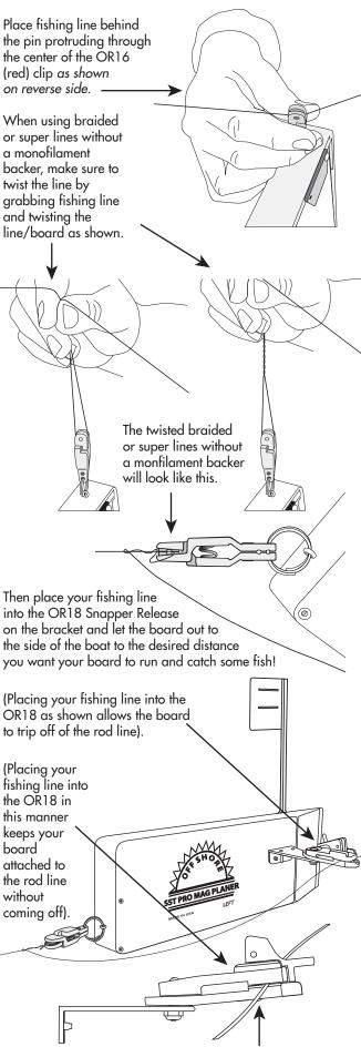
Note: To hold some lines, the tension of the OR18 may need to be adjusted. To increase tension, slightly turn the screw on the bottom of the OR18 clockwise. Small increments can make a big difference; do not over tighten.
