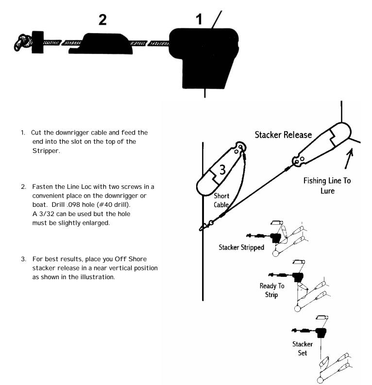
Stacking two lures on a downrigger is quicker and easier with the OR6 Stacker Stripper.
